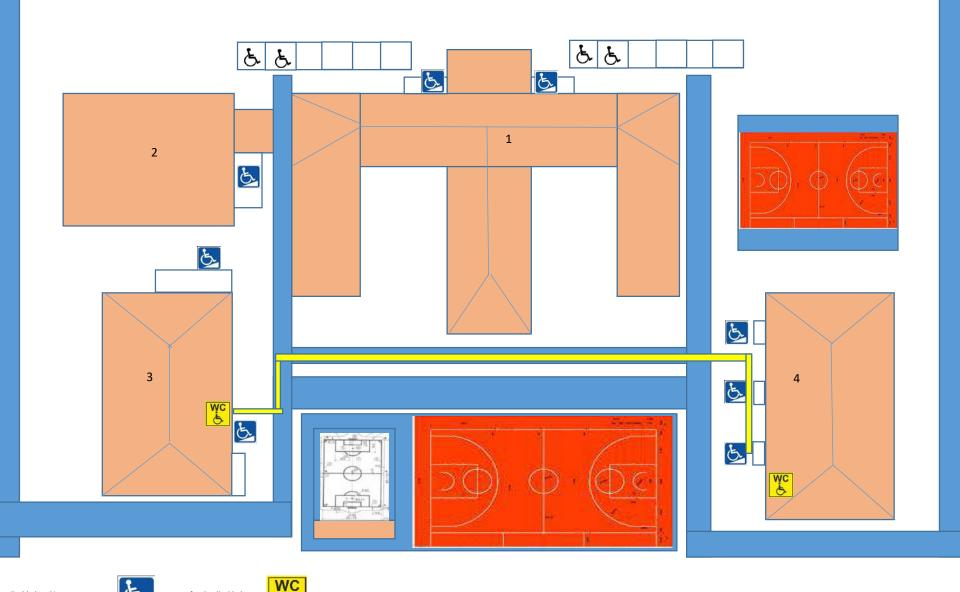
1. The main building has two ramps on both sides of the staircase. The building's staircases also have ramps. In front of the main building there are two parking lots with parking spaces for the disabled. Two spaces on each side, a total of 4 spaces.
